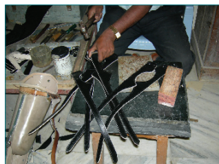
Figure 6: Production of below knee prostheses
